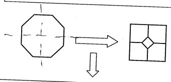
VII. Drill press the ends so the sections can be connected with thick, hollow dowels
